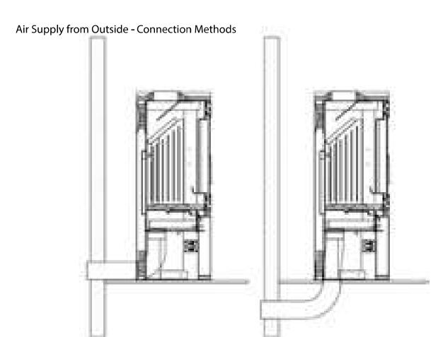
Air can be supplied to the combustion chamber from within the room or from outside. The stove is fitted with an in-built outside air-intake opening - connector dia. 100 mm. The adjustment of the primary air under the fire grate is effected by means of a single control device below the firebox door. The stove is fitted with a triple combustion-chamber air-feed system, with primary and secondary airs.
